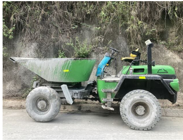
Photo 23: Tunnel spoil dump truck, losing oil
