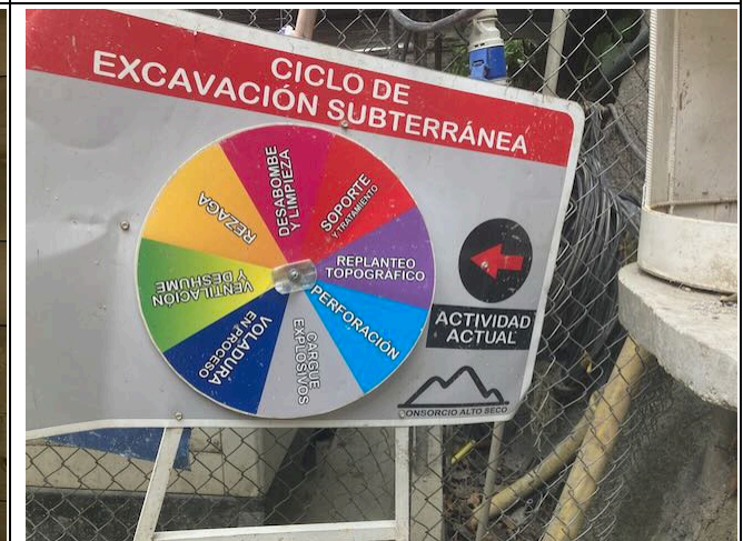
Photo 36: Signage for current stage of tunnelling activities
